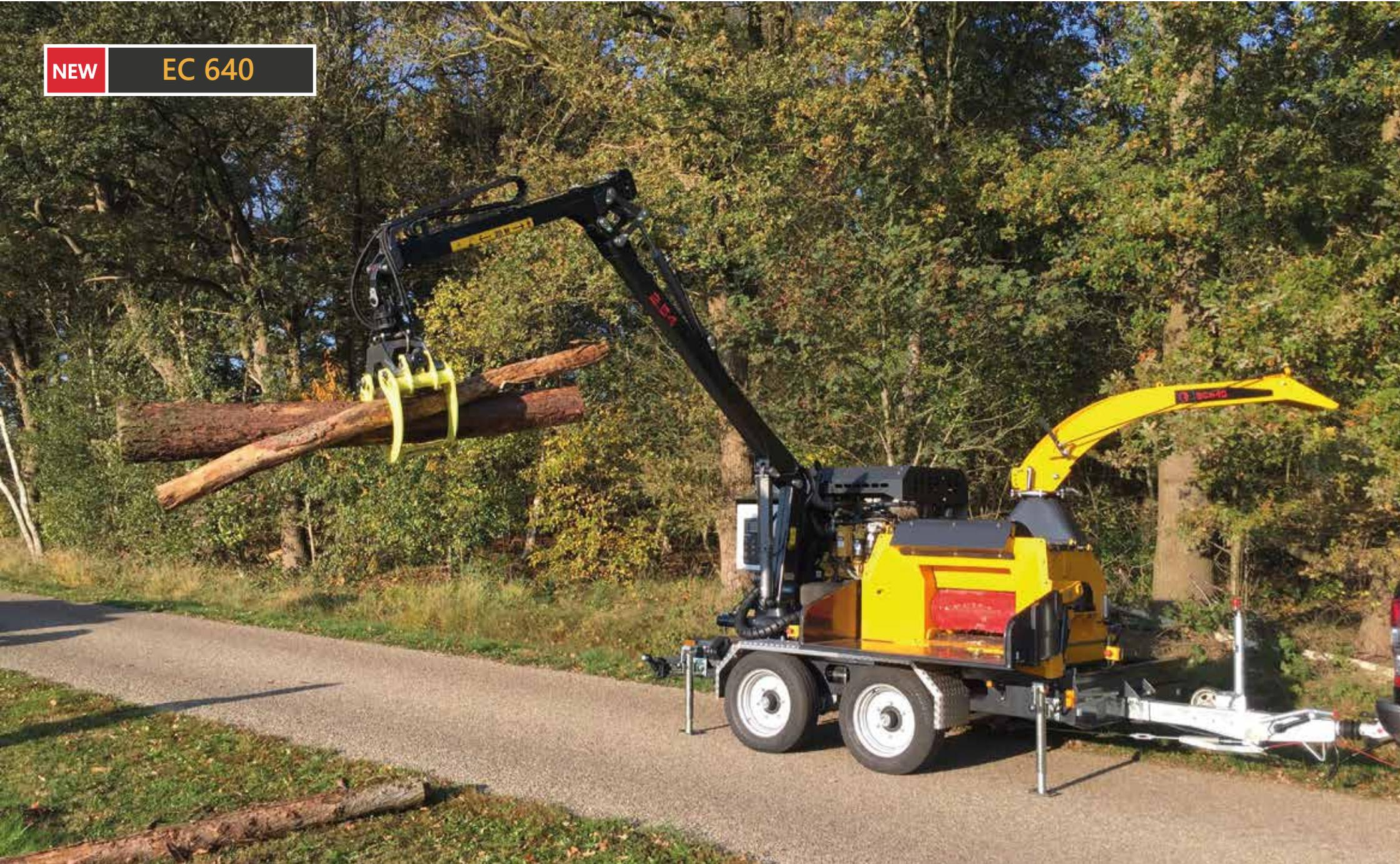
UP TO 70 M<sup>3</sup>/H. UP TO 150 HP. UP TO 400 MM LOGS.
