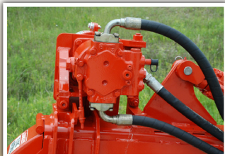
HYDROSTATIC DRIVE With 4.6 ci hydrostatic motor, 8cc gear pump and 2.48 ci hydrostatic transmission
