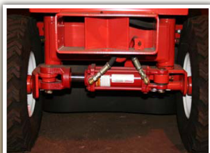
ARTICULATING FRONT AXLE Maintains stability on uneven terrain
